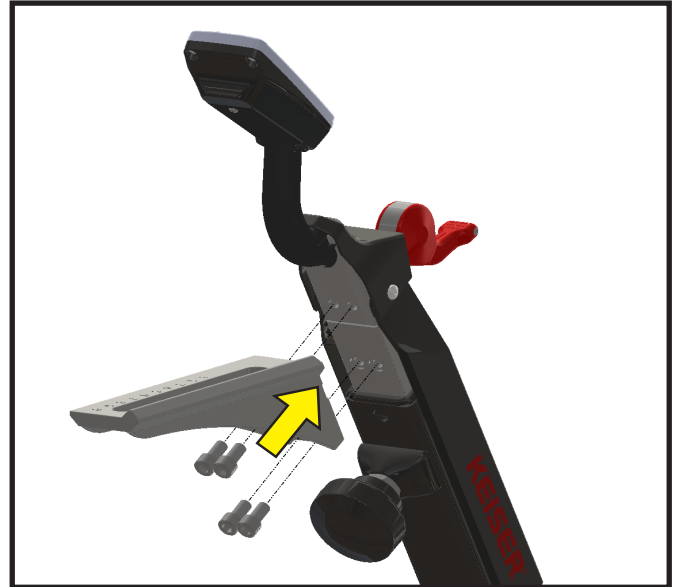
Figure 16. Attach the Bottom Slide to the Handlebar Tube
